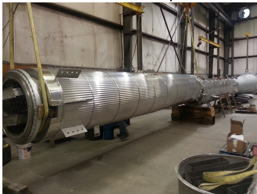
Stripper section in fabrication and assembly
