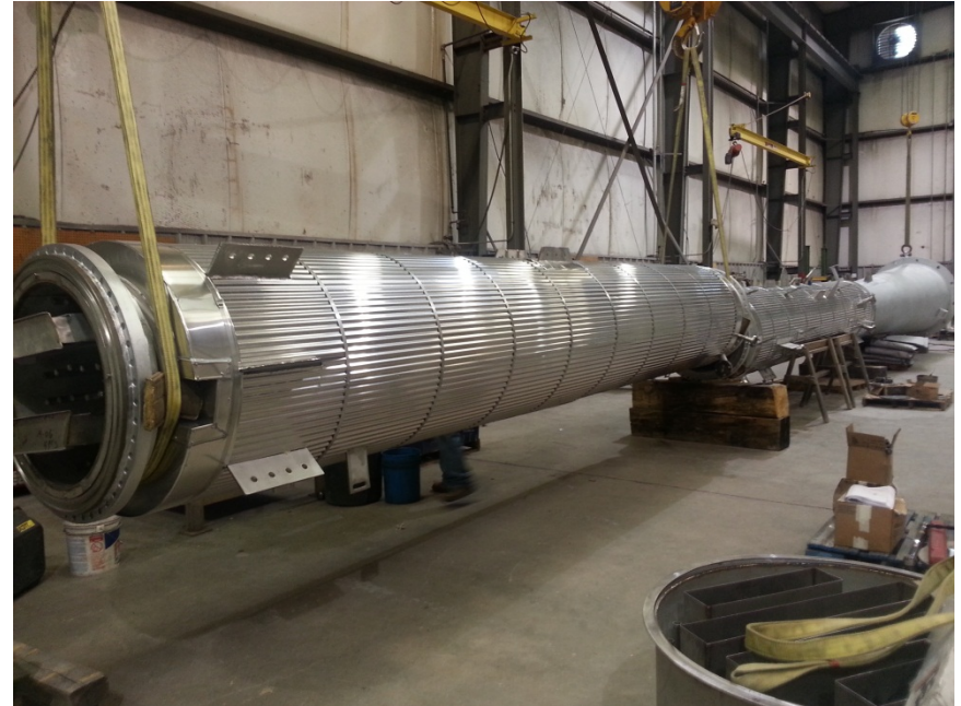
Stripper section in fabrication and assembly
