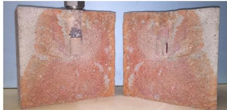
Figure 3.33: Fracture planes of Sample 27 after dyeing and gas breakdown.
