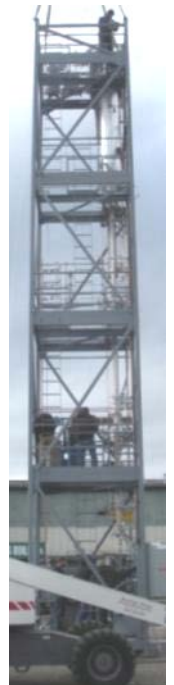
Sorbent pilot unit developed by ADA, Inc.
