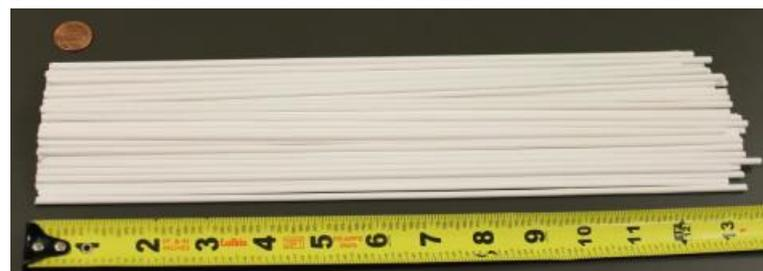
Novel  $\alpha\text{-Al}_2\text{O}_3$  hollow fibers
