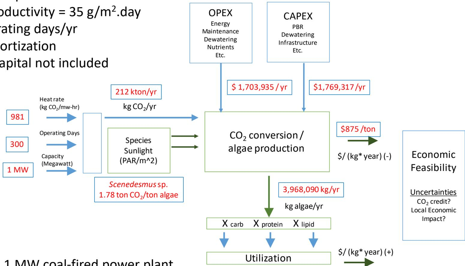
Base case: 1 MW coal-fired power plant
