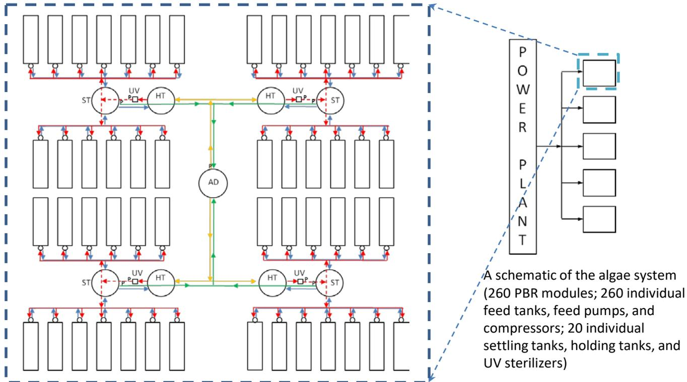
Schematic of a section of the algae system consisting of 52 PBR modules, 4 settling tanks (ST), holding tanks (HT), and UV sterilizers (UV).
