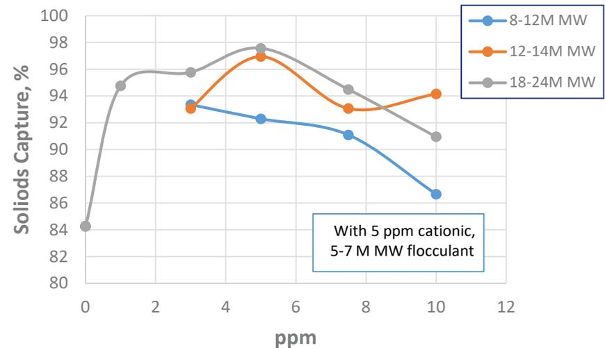
Effect of anionic flocculant dosage and molecular weight on solids capture of harvested algae pretreated with 5 ppm cationic flocculant
