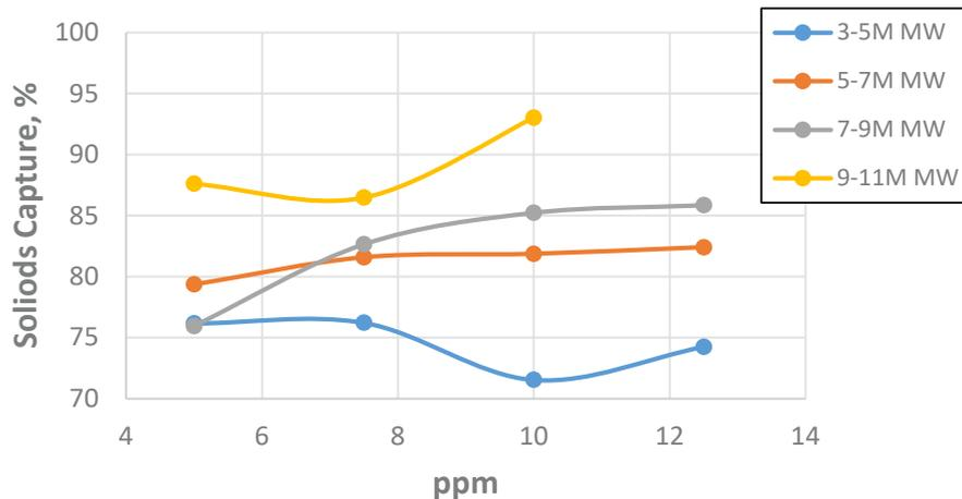
Effect of cationic flocculant dosage and molecular weight on solids capture of harvested algae (0.456 g/L)
