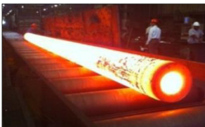
Inconel®740H Pipe after Extrusion at Wyman-Gordon
