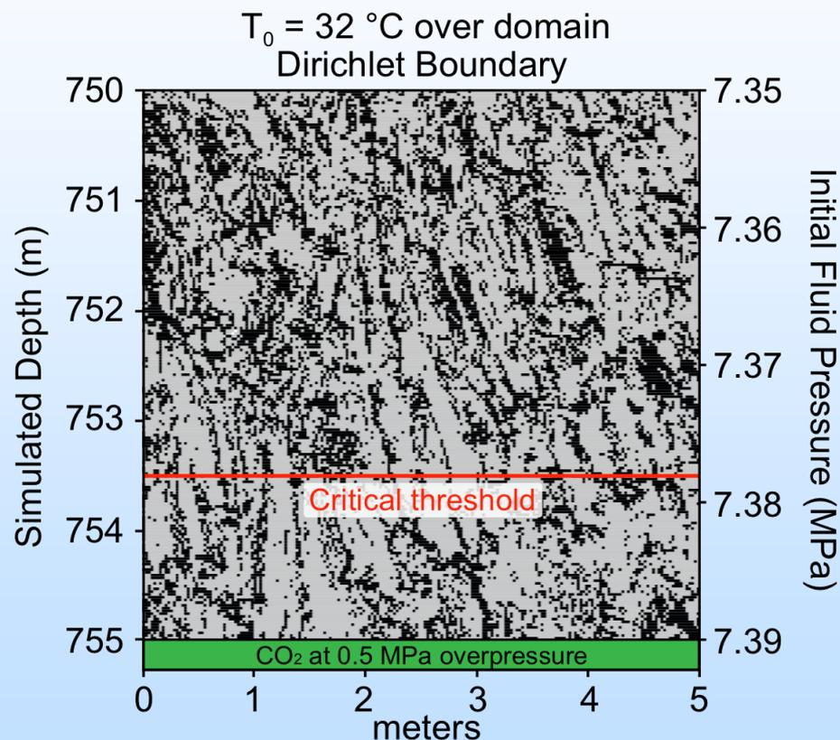
Numerical simulations with TOUGH3 (beta) and equation of state module ECO2M.
