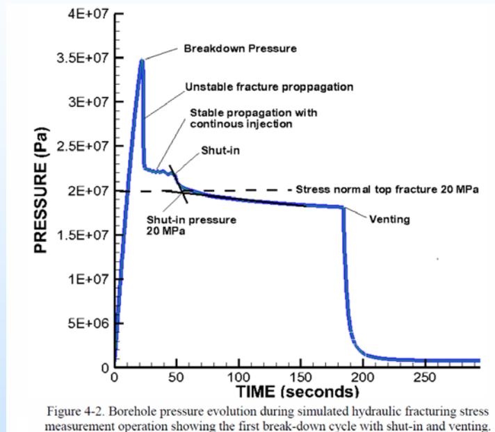
Figure 4-2. Borehole pressure evolution during simulated hydraulic fracturing stress measurement operation showing the first break-down cycle with shut-in and venting.
