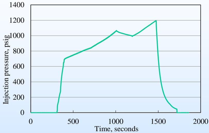
CO<sub>2</sub> injection pressure of Sample 55.
