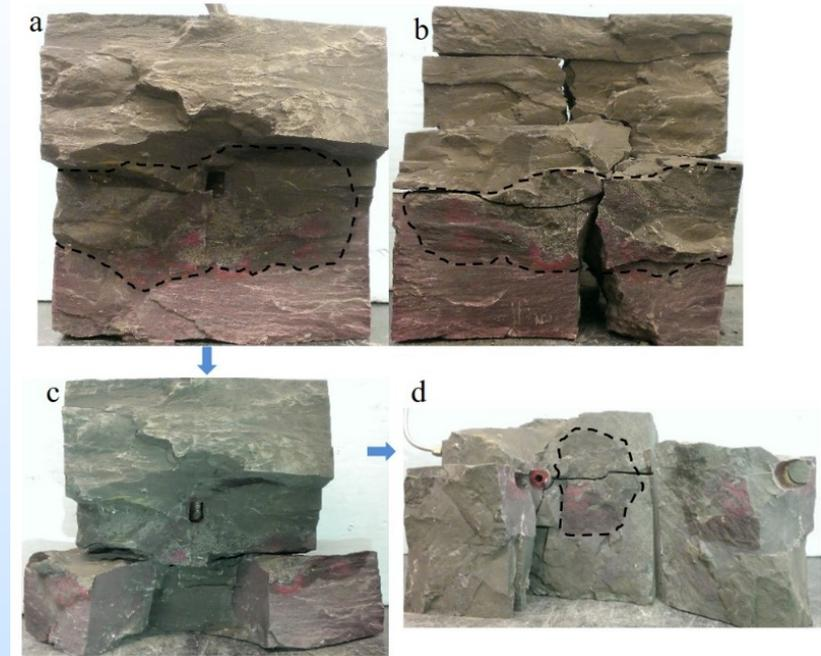
CO<sub>2</sub> injection induced fracture planes in Shale Sample 3.
