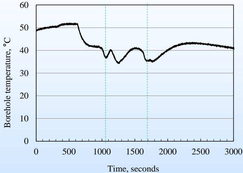
Borehole temperature profile during CO<sub>2</sub> injection into Shale Sample 3.
