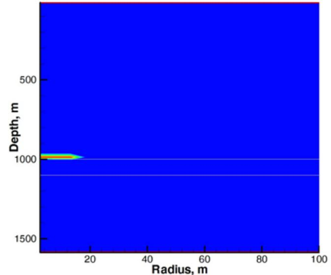
Figure 4.3. Region of caprock failure, just above the aquifer
