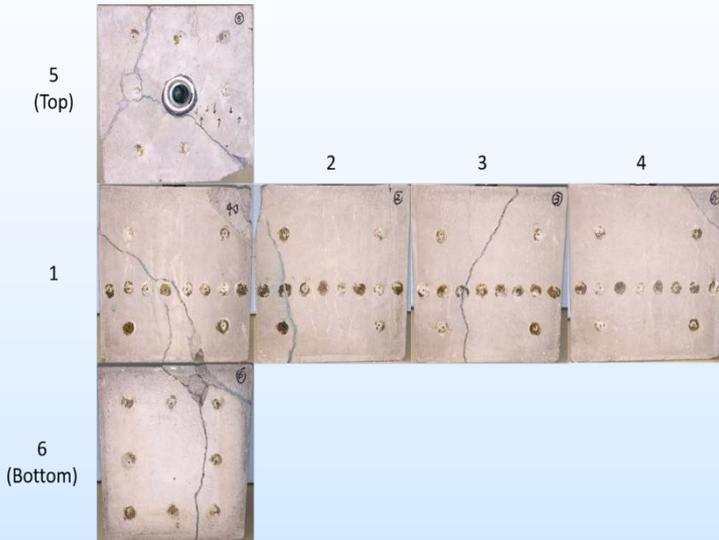
Surfaces of Sample 40 after dye and gas break-down.
