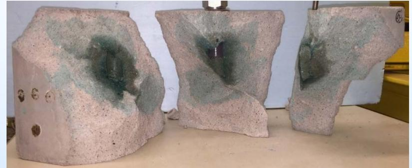
Internal fracture morphology of Sample 40 after dyeing and gas breakdown.
