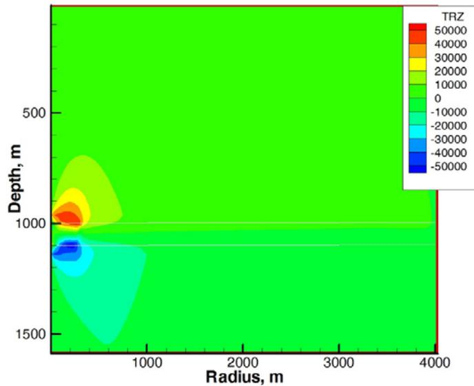
Figure 4.2. Shear stress  $\tau_{rz}$ -component after 500 days injection.
