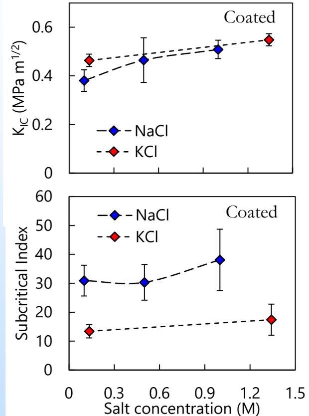
**Increase of fluid salinity increases  $K_{IC}$  and SCI in clay-rich Woodford and Mancos shales**
