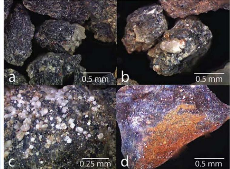
Carbonate precipitates on basalts after 854 days of reaction at 103 bar CO<sub>2</sub> and 100° C
