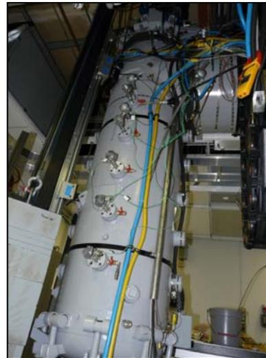
pressurized entrained flow reactor
