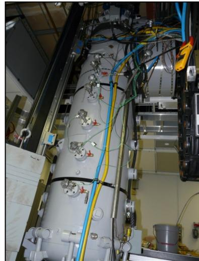
pressurized entrained flow reactor
