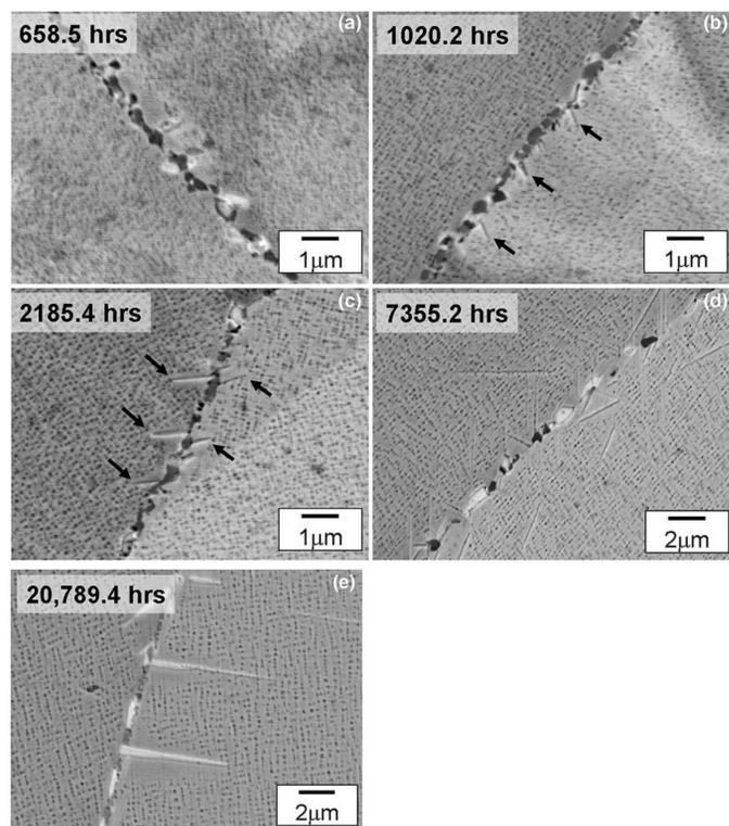
Fig. 1. Evolution of  $\eta$  phase precipitates (needle shape) at grain boundaries in Alloy IN740 exposed at 750°C. Shingledecker and Pharr, 2012.
