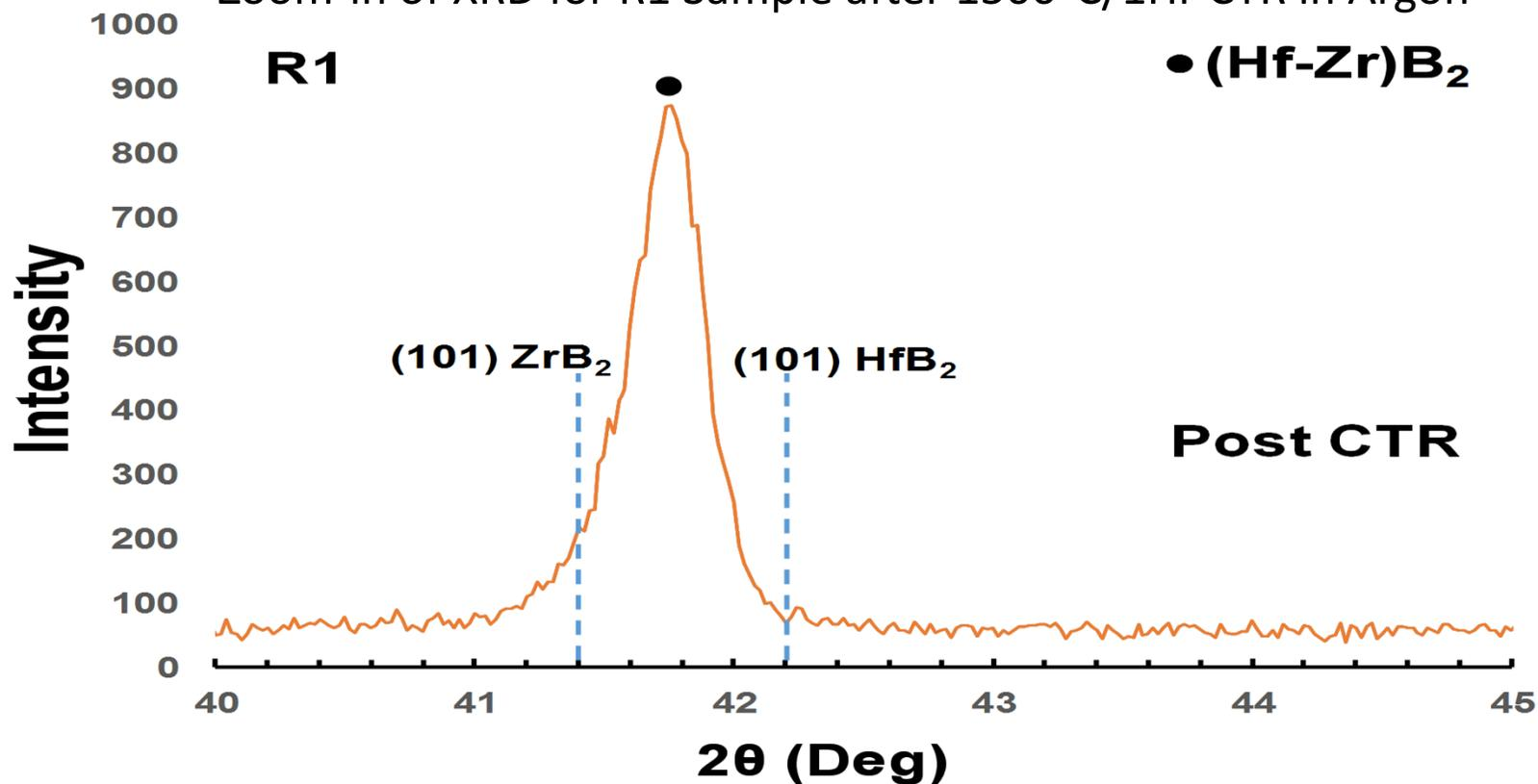
➤ (Hf-Zr)B<sub>2</sub> XRD peaks rest in-between those of pure HfB<sub>2</sub> and ZrB<sub>2</sub> confirming solid solution formation
