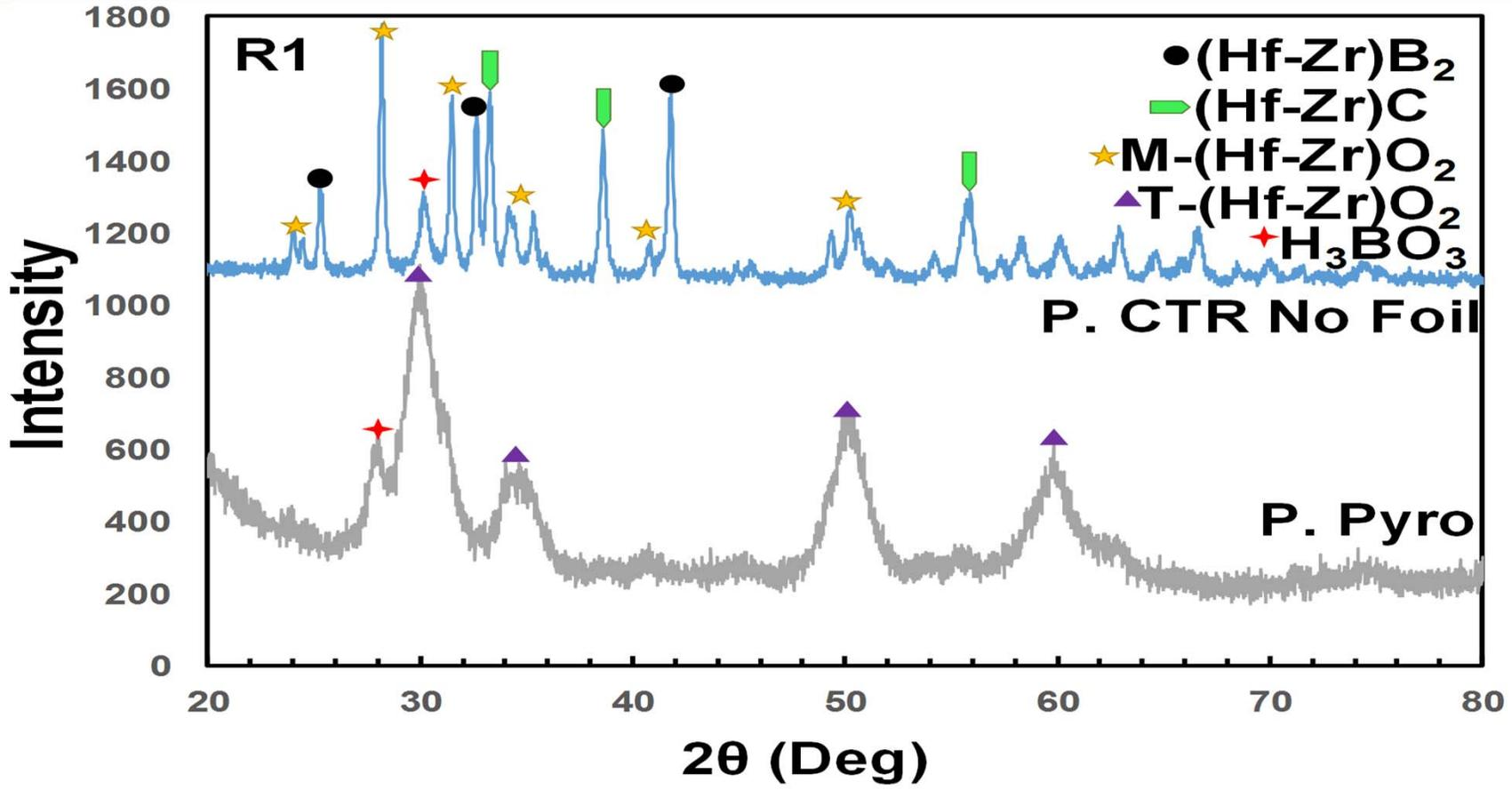
Evolution of Oxide, Boride and Carbide after CTR
