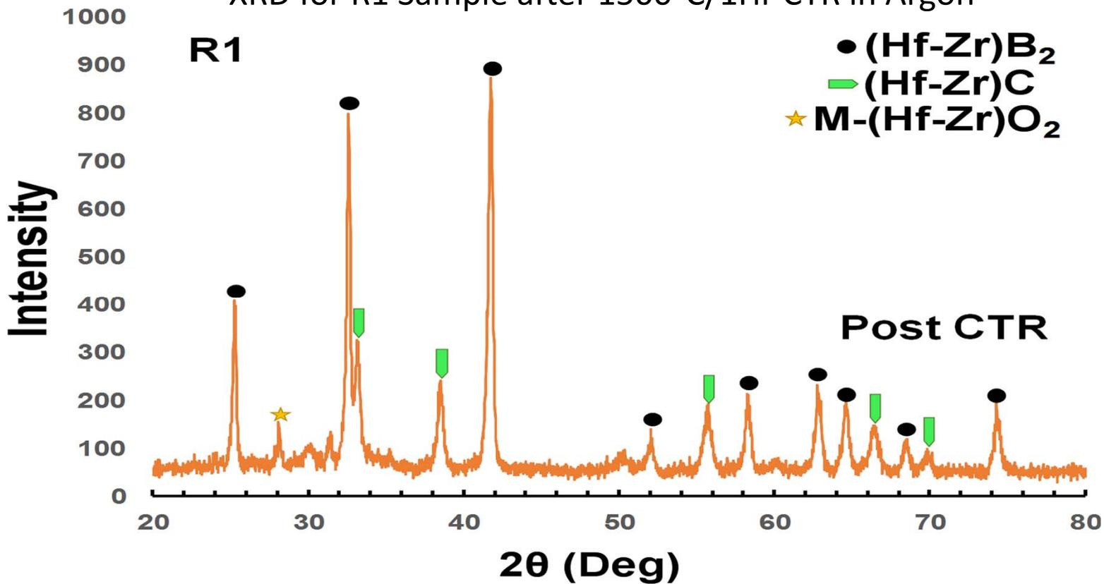
➤ Solid solution for (Hf-Zr)B<sub>2</sub> obtained
