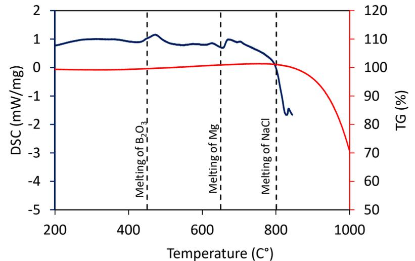
DSC and TG curves of milled mixture with 45wt% NaCl
