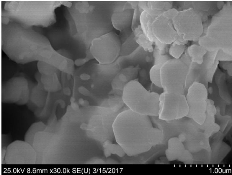
SEM Image of ZrB<sub>2</sub> obtained from a mixture without NaCl
