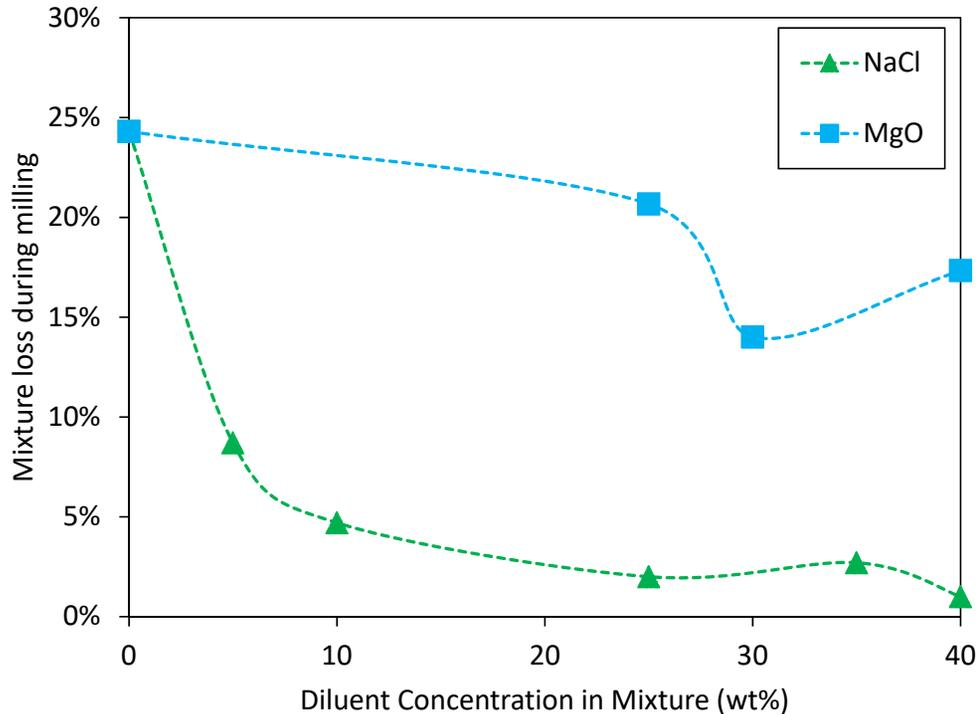
Mixture lost during milling vs. inert diluent concentration
