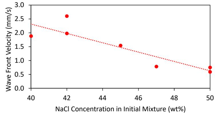
Wave front velocity vs. NaCl concentration
