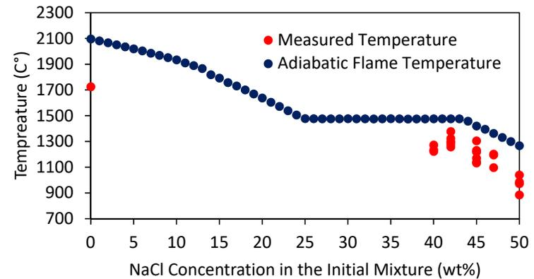
Measured temperatures and adiabatic flame temperatures vs. NaCl concentration
