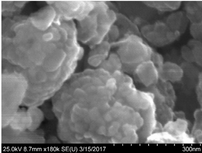
SEM Image of  $ZrB_2$  obtained from a mixture with 30 wt% NaCl and 20% excess Mg
