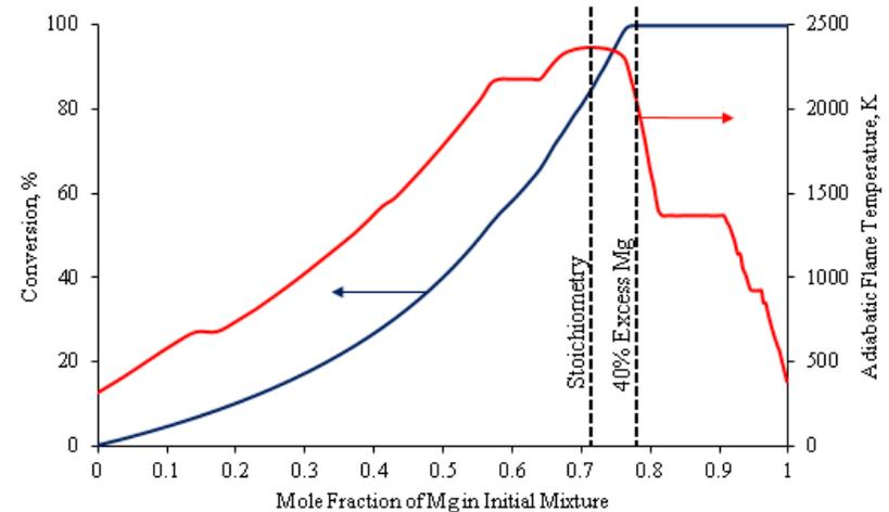
Adiabatic flame temperature and conversion % of  $ZrO_2$  to  $ZrB_2$  vs Mg concentration in  $ZrO_2/B_2O_3/Mg$  system
