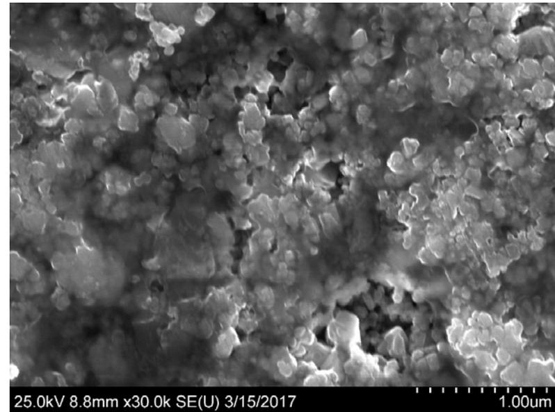
SEM Image of ZrB<sub>2</sub> obtained from a mixture with 30 wt% NaCl
