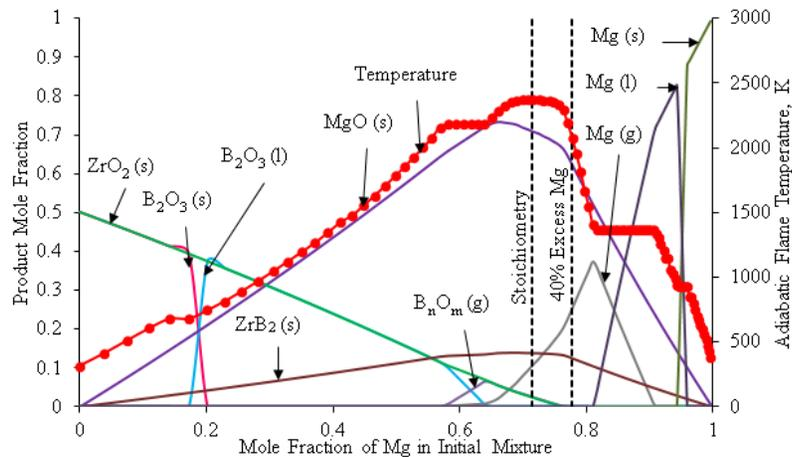
Adiabatic flame temperature and product composition vs Mg concentration in  $ZrO_2/B_2O_3/Mg$  system
