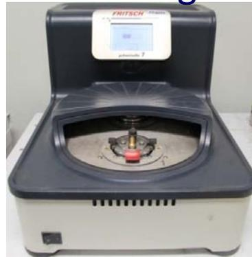
Planetary ball mill (Fritsch Pulverisette 7)
