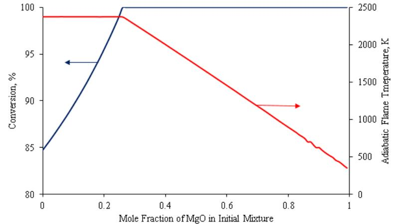
Adiabatic flame temperature and conversion % of  $ZrO_2$  to  $ZrB_2$  vs MgO concentration in  $ZrO_2/B_2O_3/Mg/NaCl$  system
