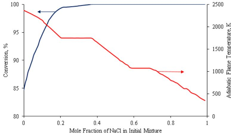
Adiabatic flame temperature and conversion % of  $ZrO_2$  to  $ZrB_2$  vs NaCl concentration in  $ZrO_2/B_2O_3/Mg/NaCl$  system
