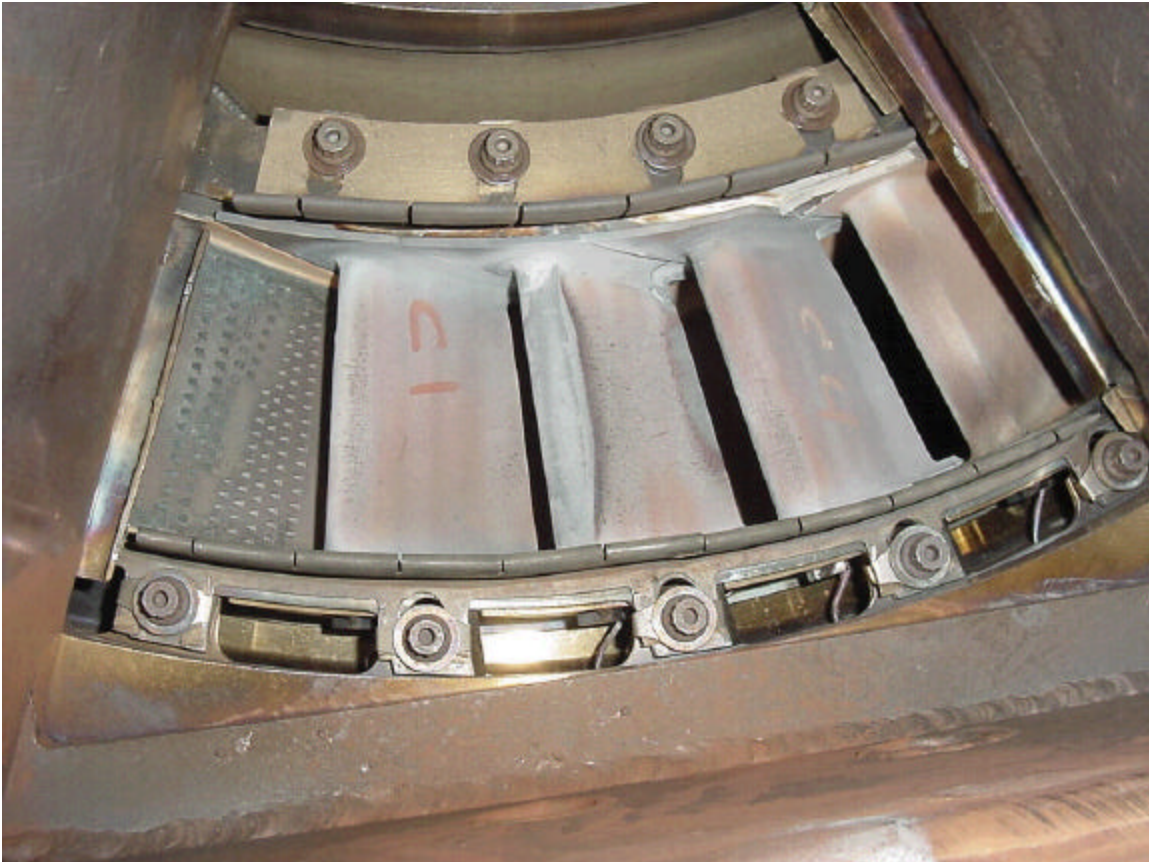
FT8 sector of cooled silicon nitride vanes with an Environmental Barrier Coating
