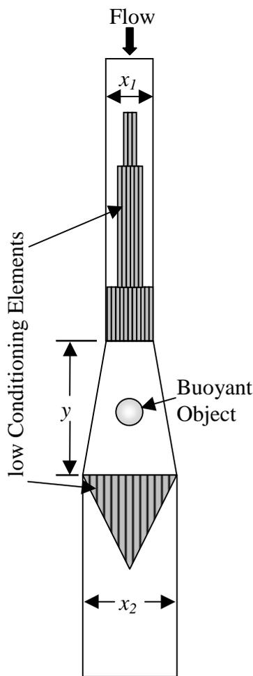
**Figure 1.** Schematic diagram of a water tunnel device
