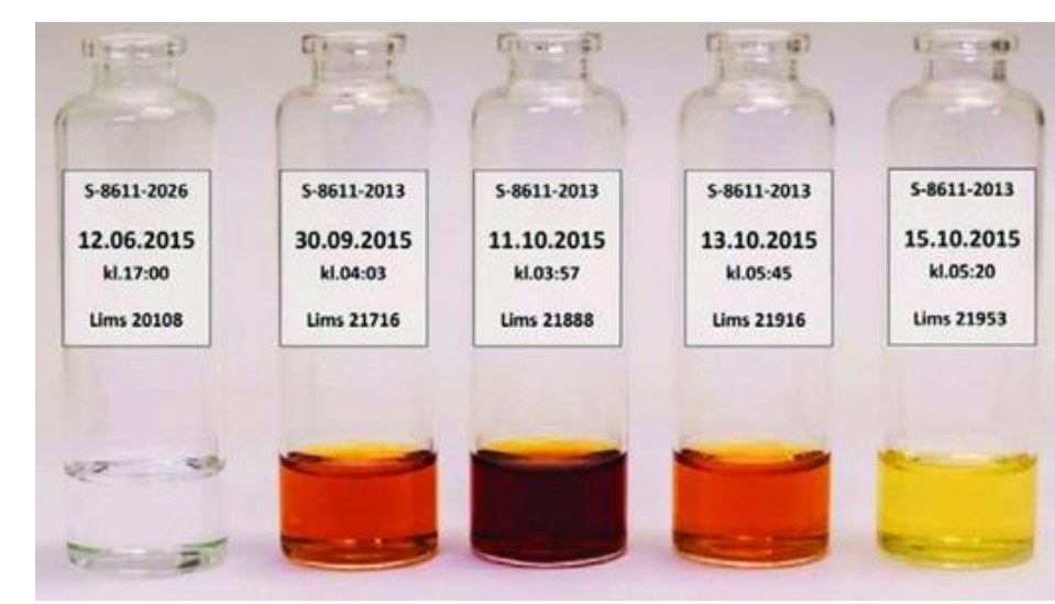
Figure 2. Examples of an amine solvent system degradation over time. 9
