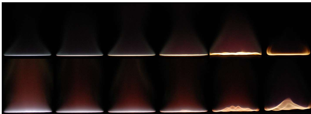
Figure 15. H 2 /NH 3 (top row), CH 4 /NH 3 (bottom row) flat flames, 30-80% by volume NH 3 (left to right), 5 slpm total fuel flow
