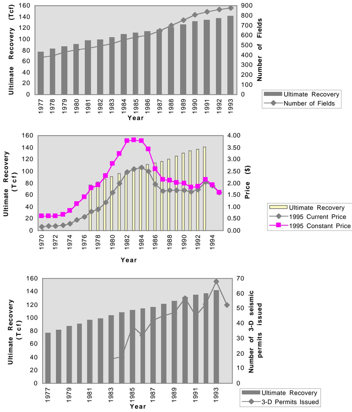
Figure 4. Natural gas reserve appreciation in GOM OCS versus field number, price, and 3-D seismic permits (Data from EIA, 1995 & Francois, 1995)
