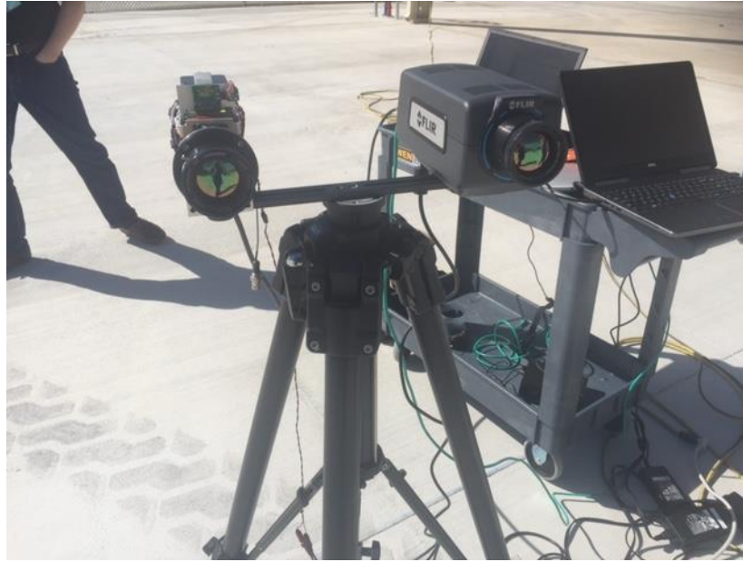
Figure 2: Niatros™ and FLIR MWIR Cameras Acquiring Data During a Supervised Methane Release
