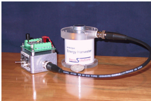
Figure 8. Demonstration unit powering Millennial Net’s [12] i-Bean wireless transceiver (see on right).
