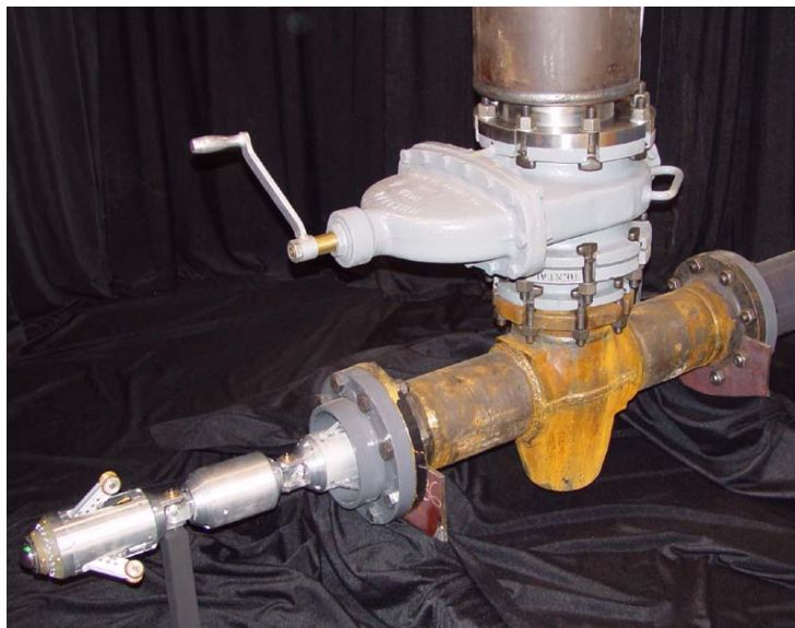
Figure X : X-I prototype in vertical launcher used for medium-pressure (< 125 psig) deployments
