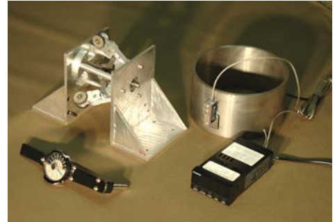
Figure L : Drive-arm strain-gauge and leg-expand/-collapse test-jig
