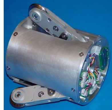
Figure LVI : Prototype Support-module of the X-II prototype tractor/train
