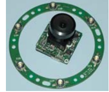
Figure XLIX : Prototype LED illuminator ring and test-camera setup
