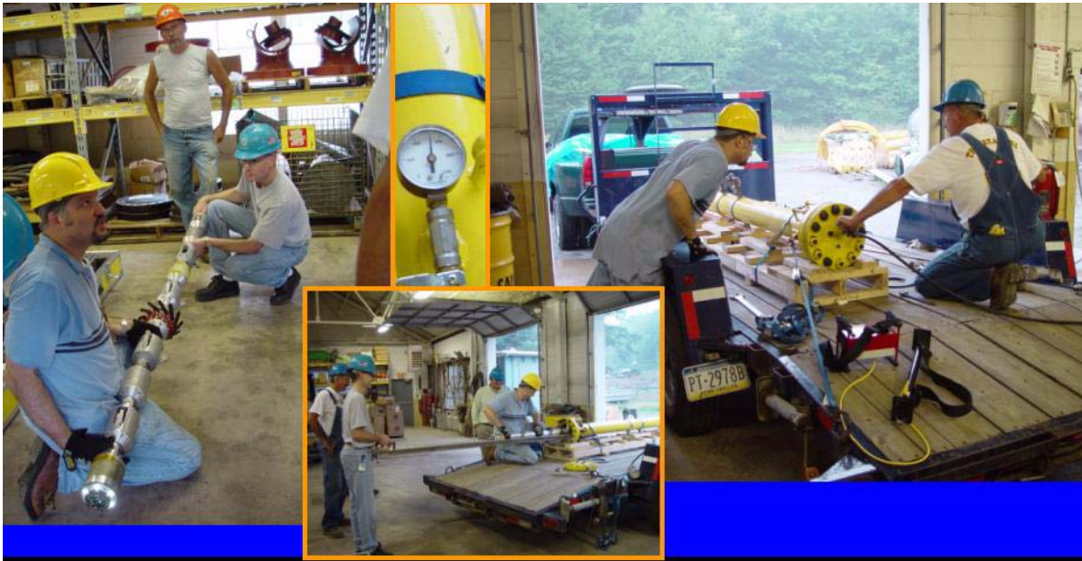
Figure LXX : Test setup of the operational and safety testing for X-II in high-pressure natural gas
