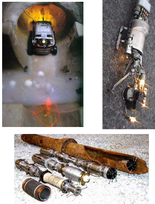
Figure XII : Tethered gasmain (CISBOT - right; GRISLEE - bottom) and untethered autonomous (Kurt I) robots developed to date by industry and researchers
