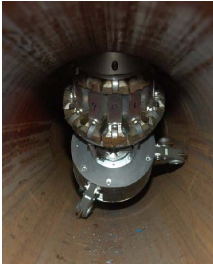
Figure LXXXIV : X-II-MFL ascending the 45-degree inclined launcher-fitting with (collapsed) MFL attached
