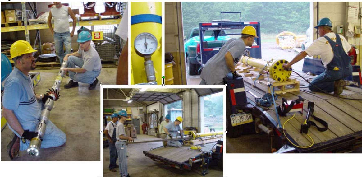
Figure V : Safety testing of X-II platform and launch/recovery procedures in pressurized (750 psig) natural gas with a participating utility at a pumping station
