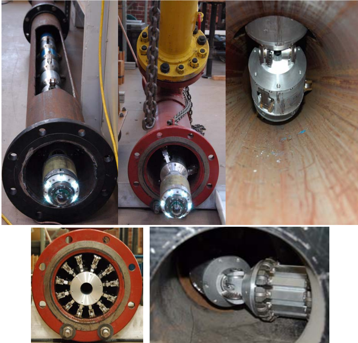
Figure LXXVIII : Typical test-setup for the MFL sensor train, including launcher, pipes (whole & cut-outs) and elbows/Ts
