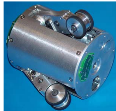
Figure LV : Prototype Drive-module of the X-II prototype tractor/train
