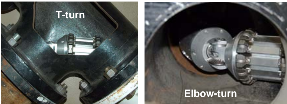
Figure LXXXIII : X-II-MFL performing a 90-degree T- and elbow turn with (collapsed) MFL attached
