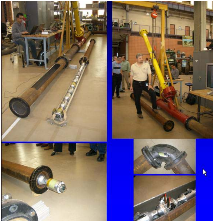
Figure LXVIII : Selected images from the X-II acceptance demonstration at CMU, depicting the robot, launcher, elbow- and T-turn, as well as sensor-operation and live wireless driving and sensor-data GUI
