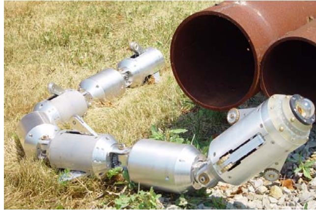
Figure IX : Explorer-I (X-I) system prototype served as a baseline platform and design for the enhanced Explorer-II (X-II) platform design and prototype
