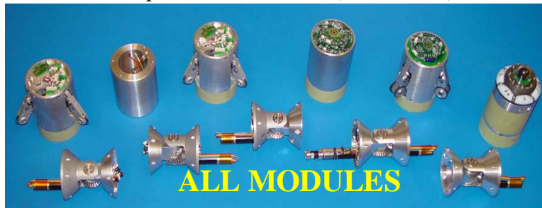
Figure LVIII : Prototype module elements for the X-II robot train/tractor
