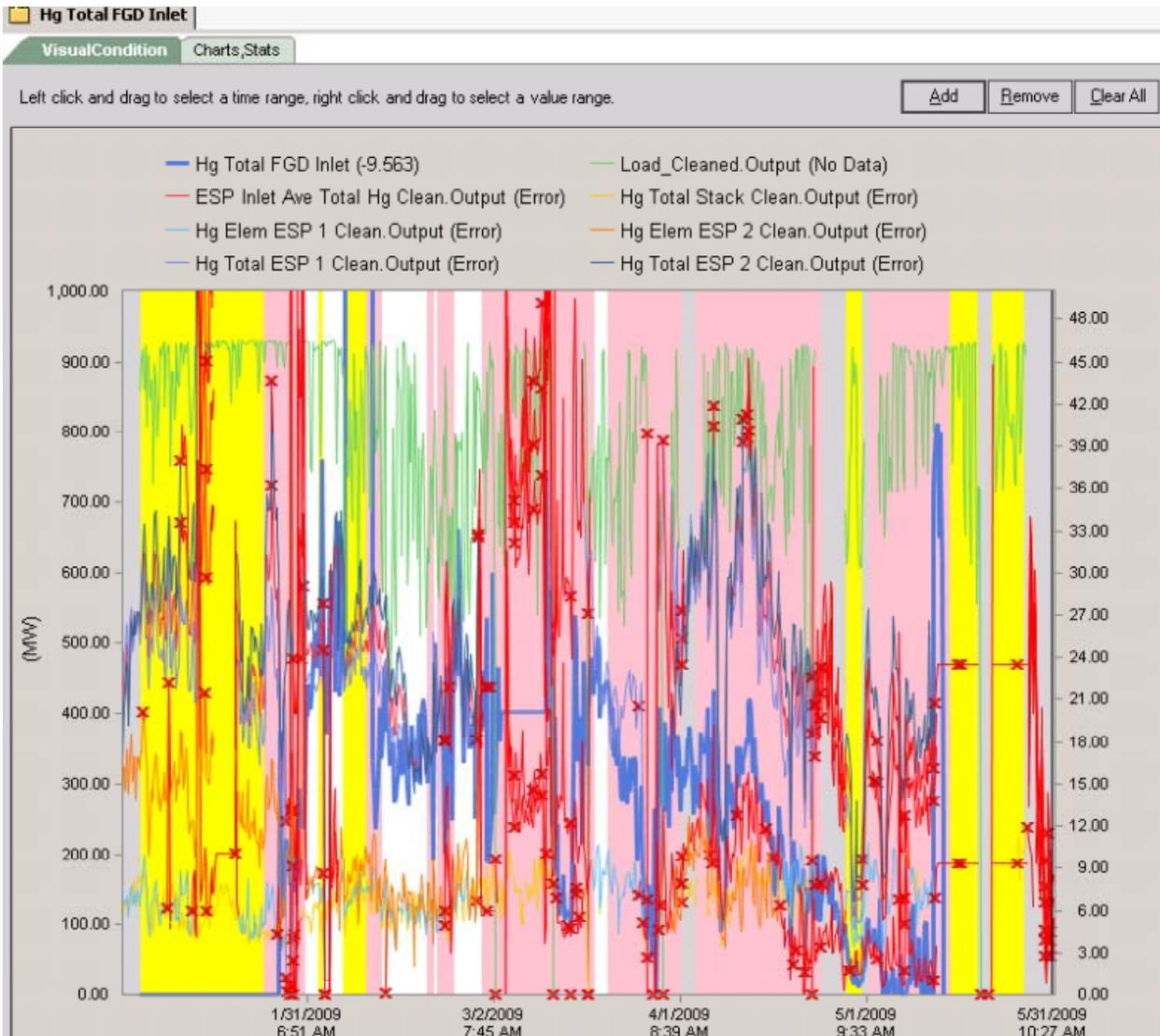
Figure 8. Total Mercury at the FGD Inlet (solid blue line) and other variables of interest. 1/1/2009 – 5/31/2009 (Ref. 1)
