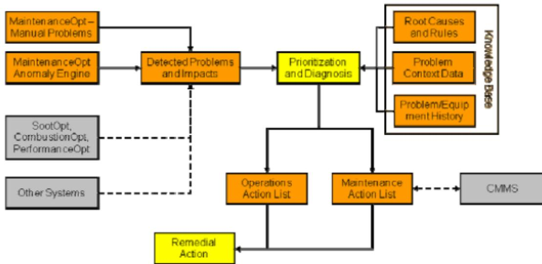
Figure 6. MaintenanceOpt Workflow for Problem Detection, Diagnosis, and Resolution (Ref. 1)
