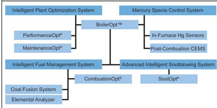
The Mercury Specie Control System included the boiler area optimization system (BoilerOpt™), in-furnace laser sensors that provided real-time information indicating species compositions and temperatures directly within the combustion zone, and CEMS at the ESP inlets, an FGD inlet and outlet, and the stack.
