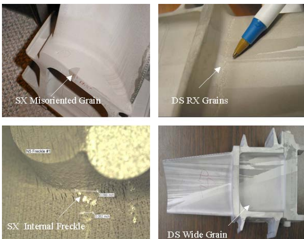
Fig. 4. Typical grain defects in SX and DS airfoil alloys that negatively impact casting yields. (Courtesy of General Electric Company).
