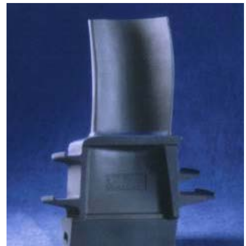
Fig. 3. First stage IGT bucket made from SX Rene' N5. (Courtesy of General Electric Company).
