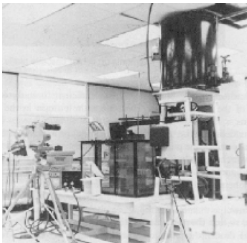
Fig. 42. Apparatus for testing axial-flow cascade model
