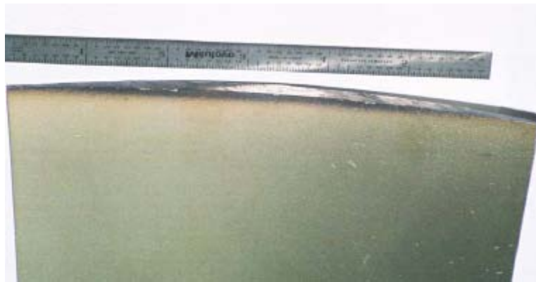
Fig. 38. Compressor Blade with Tip Rub
