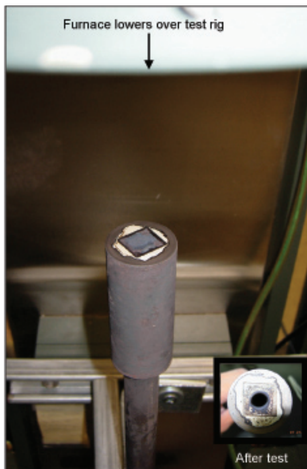
FIGURE 3. Test Apparatus Used for Measuring Burst Strength of Glass Seals at Elevated Temperature; the Bottom Insert Shows the Seal Bond Area after Rupture
