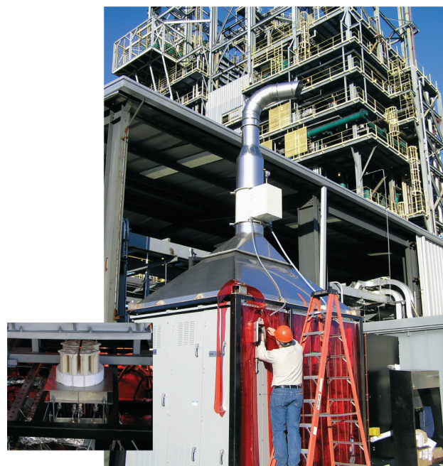
FIGURE 1. Multi-Cell Test Rig for Direct Coal Syngas Testing at the Power Systems Development Facility at Wilsonville, AL
