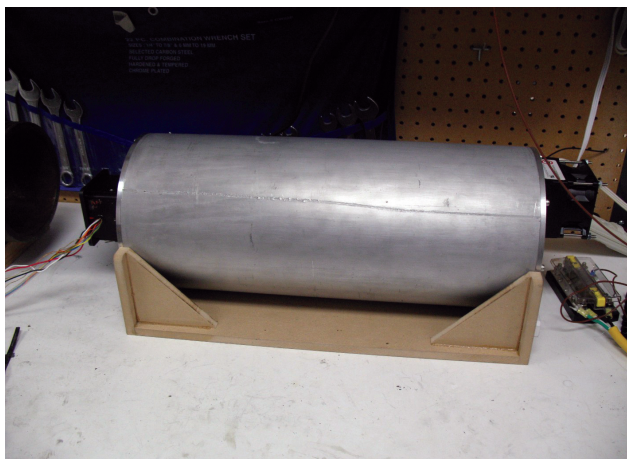
FIGURE 4. Impeller Burst Rig for Impeller Life Extension
