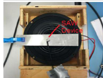
Schematic and photograph of test setup for interrogation of LGS SAW resonator under dynamic stress conditions.
