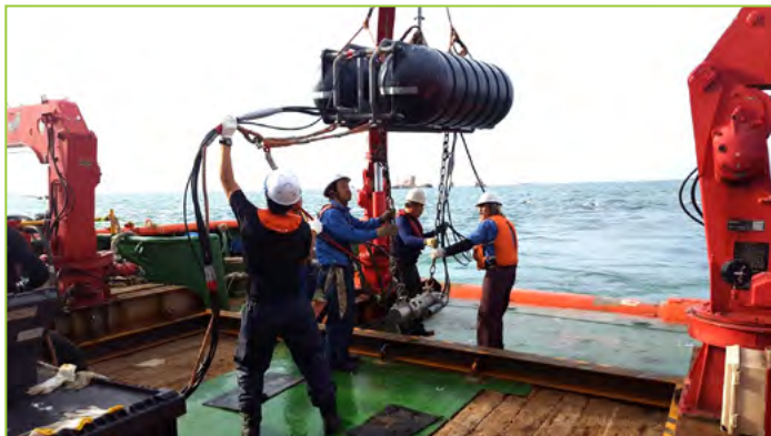
Acoustic energy sources (compressed air) being deployed for ultra-high-resolution 3D seismic data acquisition at the Tomakomai CO 2 storage demonstration project offshore Tomakomai, Hokkaido, Japan.
