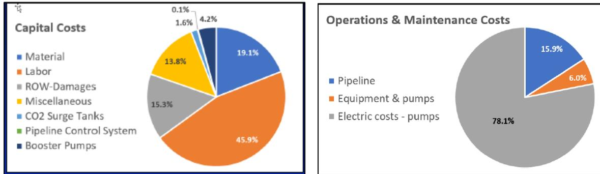
Figure 7. Estimated break up of pipeline costs associated with capital and O&M (source: McFarlane and Dubois, 2017).
