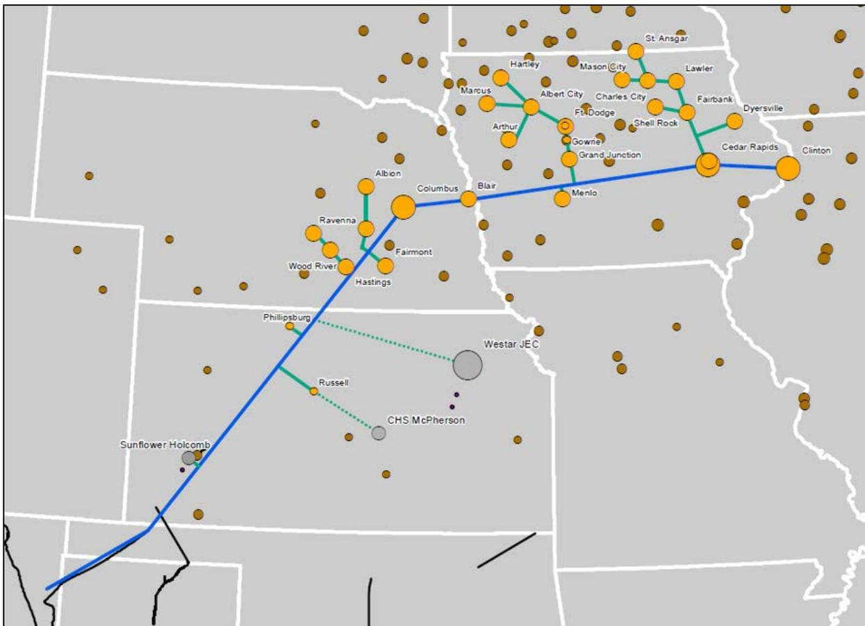
Figure 10. Location of CO<sub>2</sub> sources, receiving oil fields, and pipeline route for Scenario 3 {Symbol legend: yellow-brown (ethanol), and light grey (industrial and coal-fired electric plant)}.
