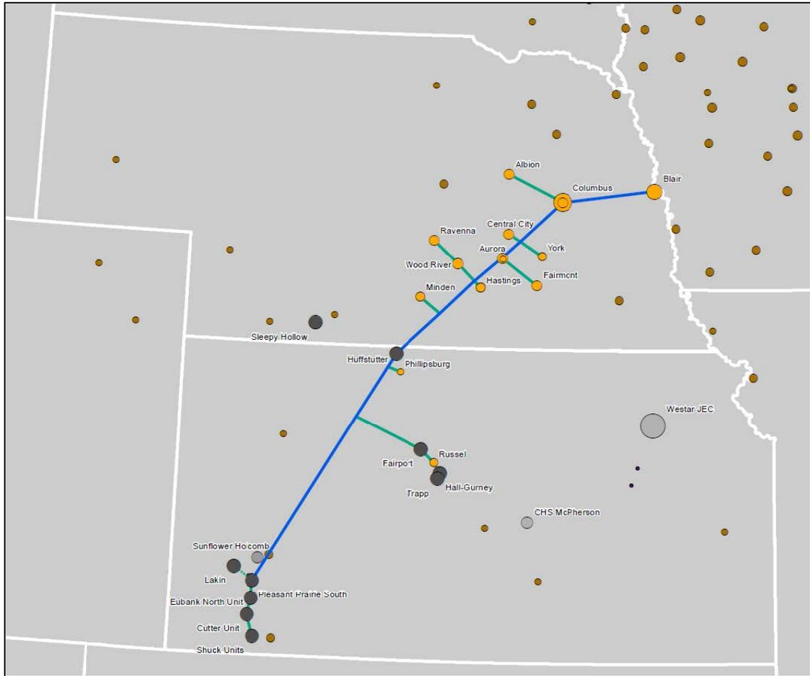
Figure 8. Location of CO2 sources, receiving oil fields, and pipeline route for Scenario 1 {Symbol legend: yellow-brown (ethanol), black (industrial), and light grey (coal-fired electric plant)}.
