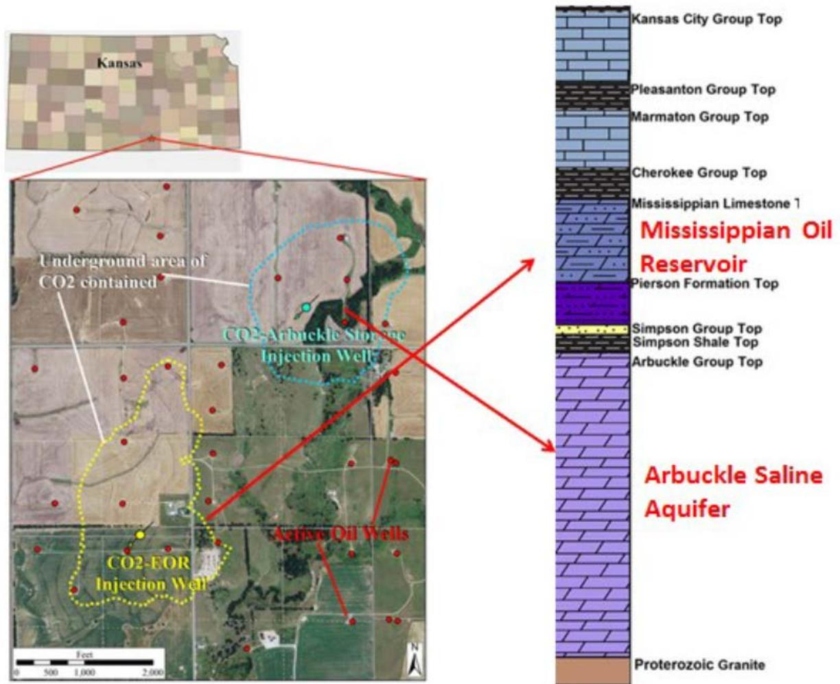
Figure 4. Location of CO<sub>2</sub>-EOR and storage pilot-scale test site at Wellington, KS.
