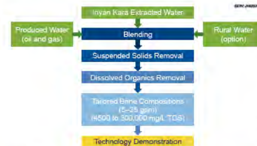
Conceptual extracted water treatment flow diagram.
