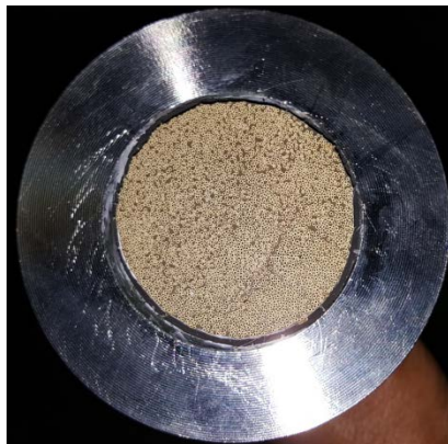
Potted 4-in fiber module cross-section (early design)
