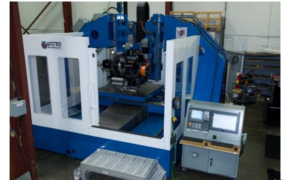
Sheet Lamination UAM Fabrisonic
