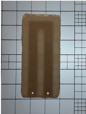
YSZ imbedded thermistor imaged over light box
