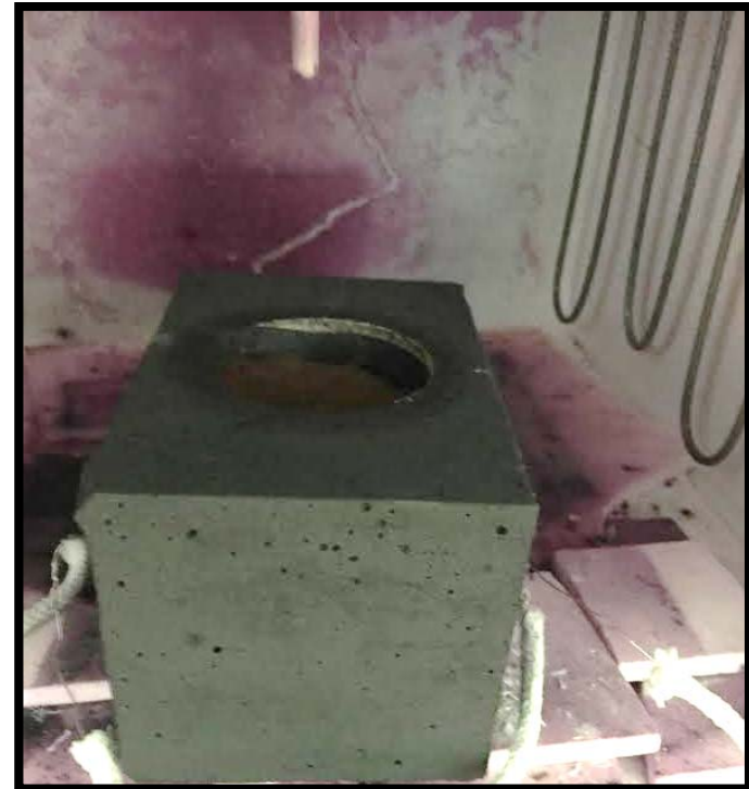
Thermistor embedded smart brick in the testing furnace
