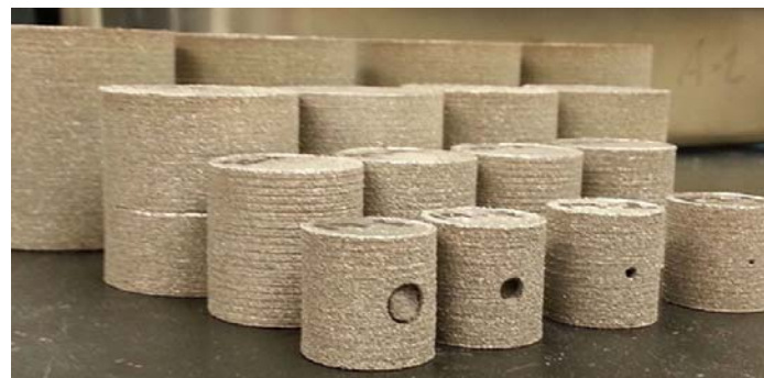
25mm cylinder (4mm channel)
