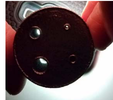
Holes after liquid nitrogen and ultrasonic vibration
