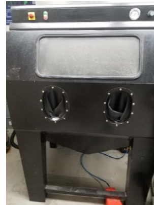
Powder Recovery System (PRS)
