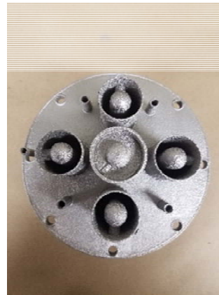
PRS applied to the large orifices, 0.218 lbs powder removed
