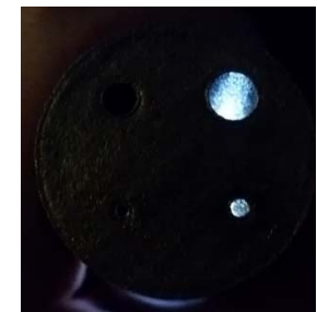
Light was shown through the holes to assess powder removal
