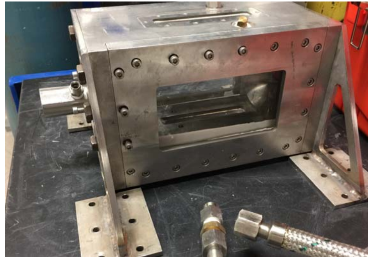
Multi-purpose Optically Accessible Combustor (MOAC)
