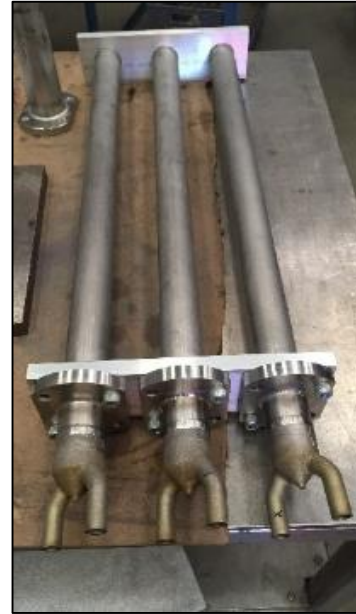
SCO 2 manifolds and in-bed heat exchanger assembly
