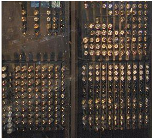
The 1946 ENIAC computer used 17,468 vacuum tubes and consumed 150 kW of power
