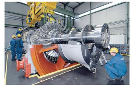
Siemens SGT5-8000H 375MW Gas Turbine
