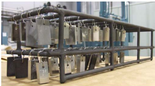
Figure 2. Test Rack with Coupons
