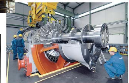
Siemens SGT5-8000H 375MW Gas Turbine
