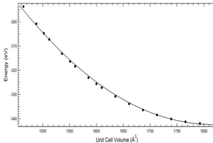
Left: The model will be used in simulation for HfNbTaTiZr. Right: The best fit solid line of the Birch–Murnaghan equation. The bulk modulus 198 GPa.
