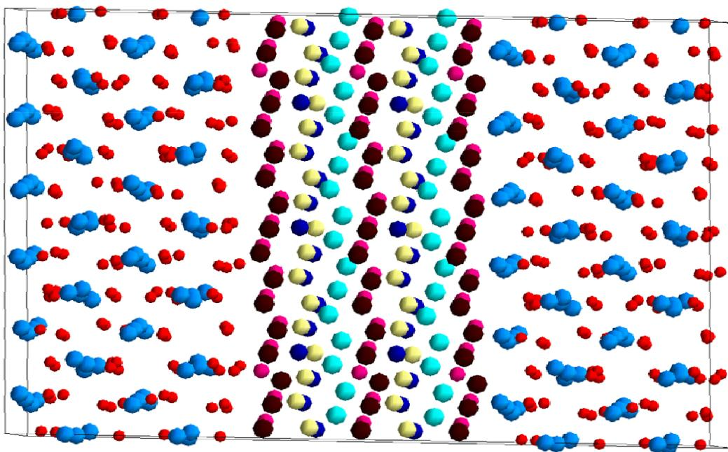
MoNbTaVW/ $Y_2O_3$  interface model: the sky blue ball stands for Y atom, red for O, light blue for Ta, yellow for Nb, pink for V, dark blue for Mo, and black for W. There are 192 Y atoms, 288 O atoms, 34 Ta/Nb/Mo, and 51 V/W with total 694 atoms are included in our tentative running interface model.
