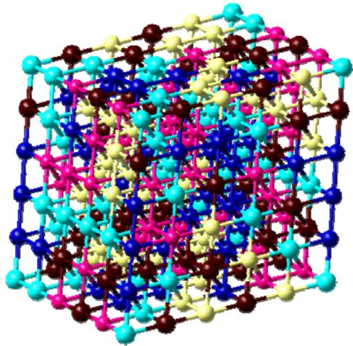
The 125 atom ball & stick special quasirandom structure model of MoNbTaVW. Dark blue balls are standing for Mo atoms, yellow for Nb, light blue for Ta, red for V, and brown for W. The initial lattice parameters are:  $a = b = c = 11.2543 \text{ \AA}$ , and  $\alpha = \beta = \gamma = 109.47^\circ$ .
