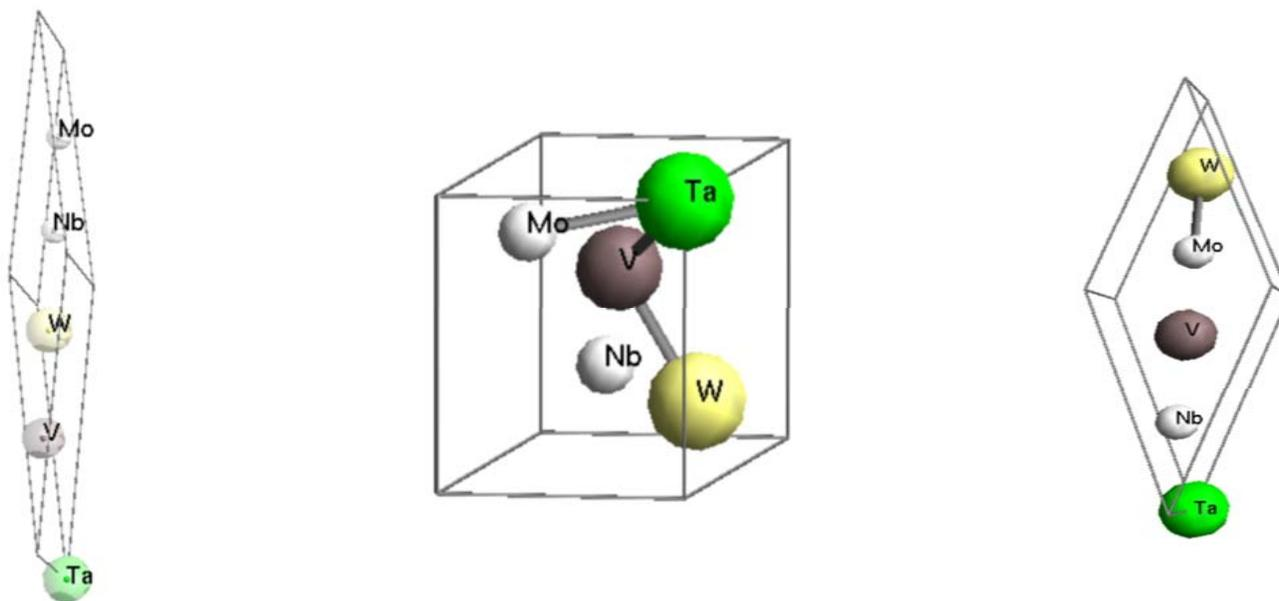
Three ordered MoNbTaVW structures were built and optimized for efficient mechanical, electronic structure, and thermal dynamics (high T) properties screening and prediction.
