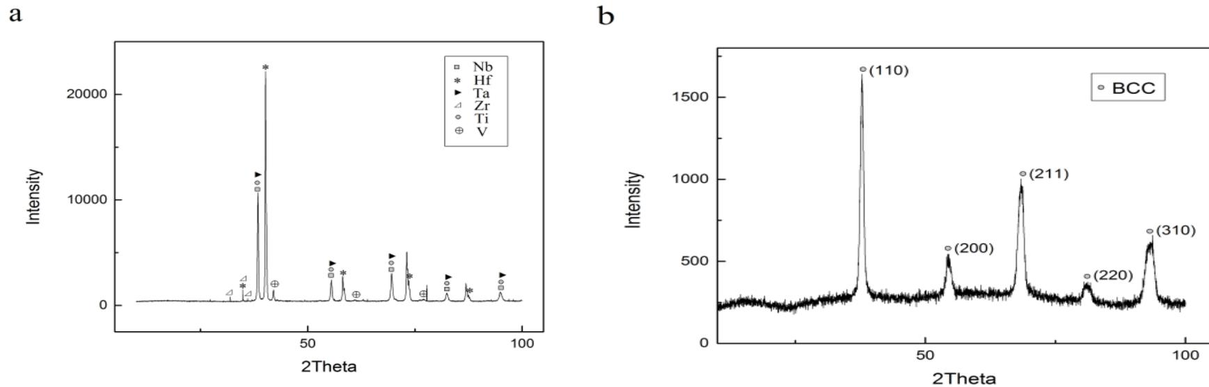
XRD patterns of HfNbTaTiVZr in the (a) pre-melting powder mixture and (b) as-solidified state
