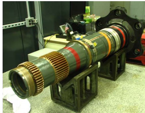
Ferrium C61 steel forward rotor shaft for Boeing's Chinook platform, 20% increase in power at same geometry vs. 9310.
