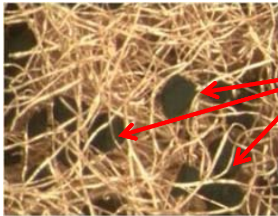
Cu-entrapped FT Catalyst Particles
