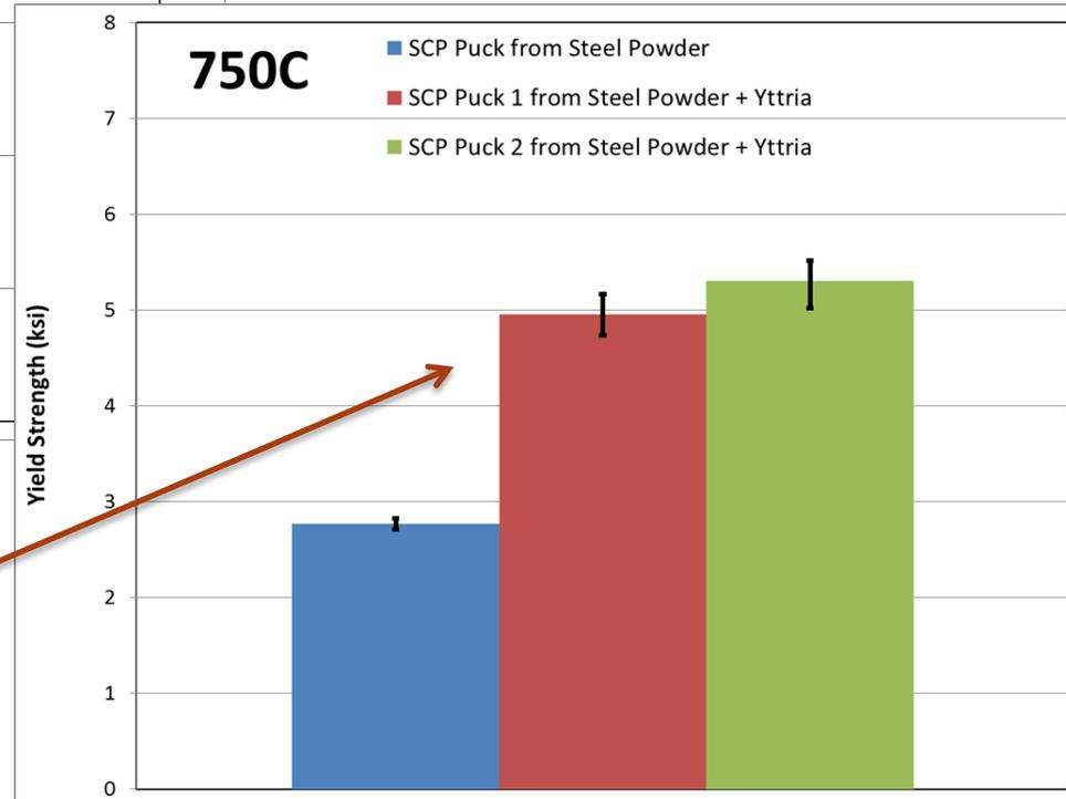
Elevated temperature yield strength is up by 72% indicating probable effect of dispersion strengthening
