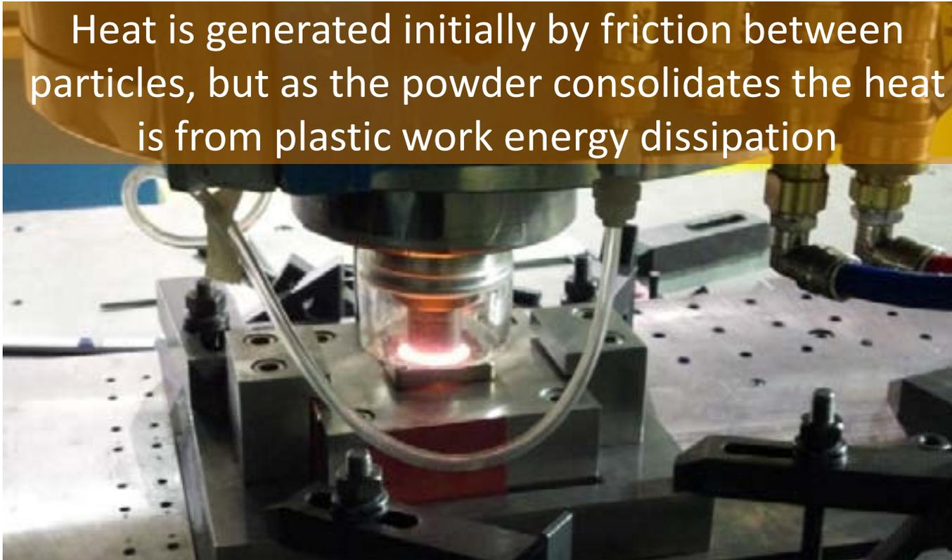
The energy released from plastic work results in significant heating, up to **700 to 900°C**. The heat and strain energy imparted to the powders causes them to fully densify and flow within the reservoir in a complex way dictated by the design of features on the face of the tool.
