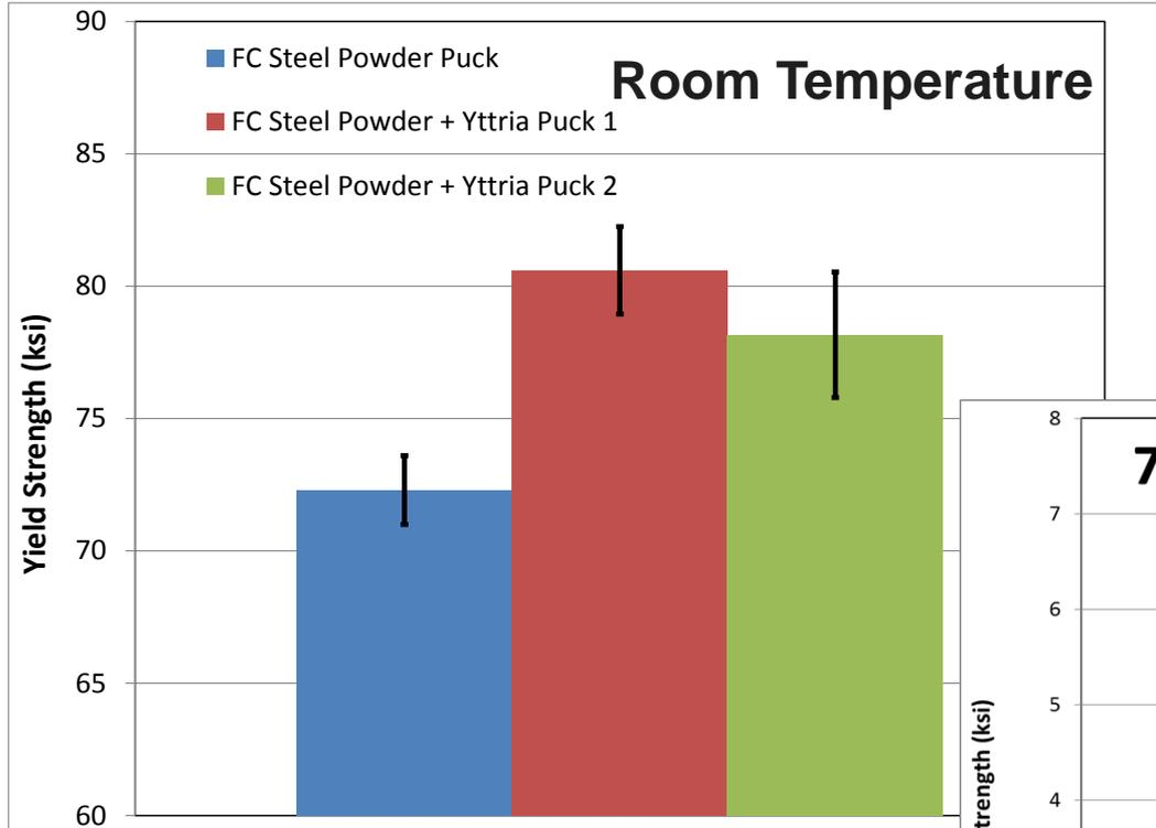
Addition of yttria and densification by FCE increases the yield strength by 6-8ksi at room temperature (8%)
