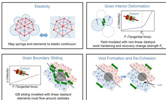
Above: Schematic representation of initial micro-mechanisms to be considered.
