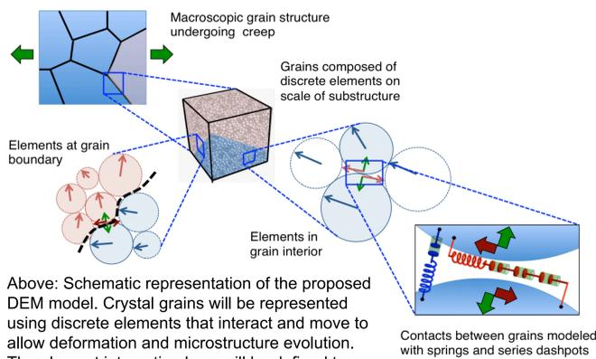
Above: Schematic representation of the proposed DEM model. Crystal grains will be represented using discrete elements that interact and move to allow deformation and microstructure evolution. The element interaction laws will be defined to represent the physical mechanisms involved for nickel based alloys
