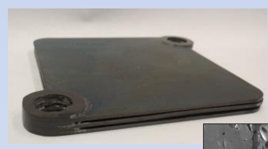
SiC to SiC - 2 micron-thick braze joint
