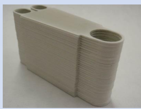
SiC to SiC - 2 micron-thick braze joint
