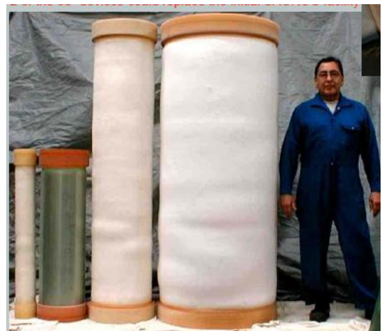
Large CO 2 /CH 4 module 76 cm OD x 1.8 m Used on 700 MMSCFD offshore platform Courtesy, E. S. Sanders NAMS 2003 plenary
