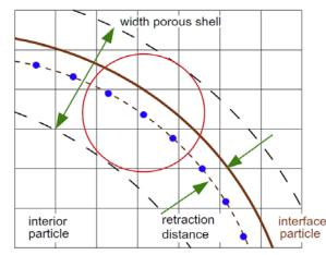
**Fig. 3.** Illustration of the porous shell covering a solid particle. The dots indicate the position of Lagrangian grid points, which are retracted from the actual interface (the solid line) with a fraction of the Eulerian grid spacing (about  $0.3\Delta x$  in this case). The circle depicts the range of action of the regularized Dirac delta function.
