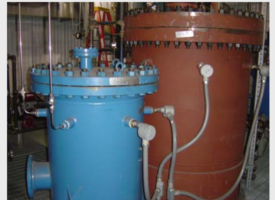
Stage II de-S & de-Cl Sorbent Feed Systems
